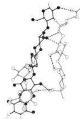
Fig 43 Xanthan gum helix with associated hydrogen bonding
