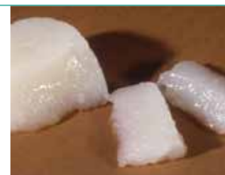
Fig 86R Indican gel formation in ethylene glycol
