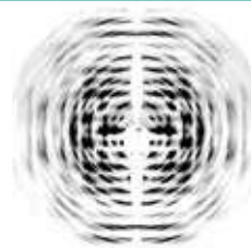
Fig 36 X-Ray diffraction diagram of cellulose
