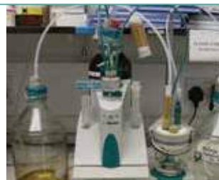
Fig 5 Karl Fischer apparatus for moisture determination
