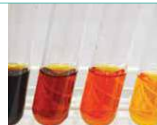
Fig 6 Use of the phenol-sulphuric test for carbohydrates (sensitivity ~ 10 µg/ml)
